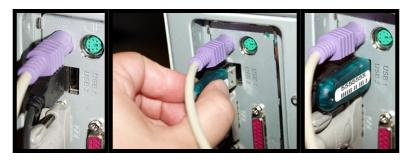
Installation of the USB Key Block
